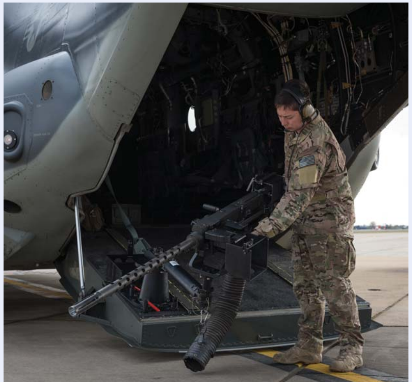
U.S. Air Force Staff Sgt. Justin O'Brien, 7th Special Operations Squadron special mission aviator, performs preflight checks on a CV-22 Osprey's ramp-mounted weapon system, a .50-caliber GAU-21 heavy machine gun Mar. 7, on RAF Mildenhall, England. When assigned to the tail position of the aircraft, SMAs are responsible for operating the RMW, weight and balance, clearing the landing zone and alternate insertions and extraction methods, among other duties. Photo by U.S. Air Force Capt Chris Sullivan.
